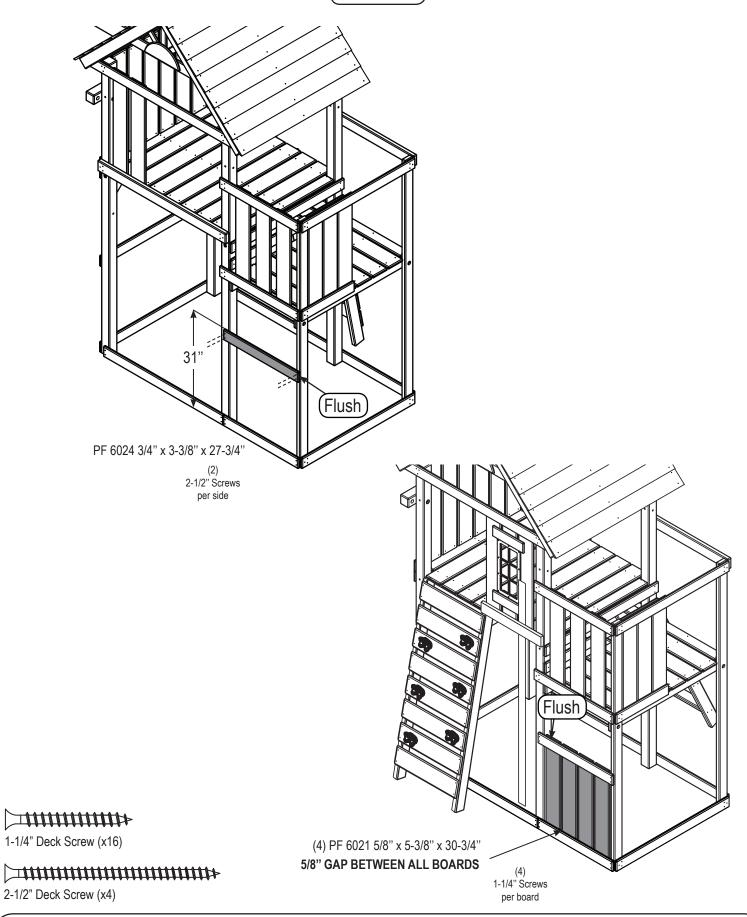
1. Install Barrier Support and Barrier Boards as shown.
