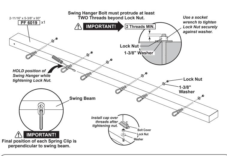
1. Attach Swing Hanger(s) to swing beam as shown.
