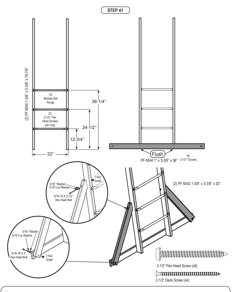
1. Assemble vertical ladder as shown.
