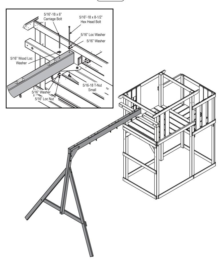
1. Install Swing Beam as shown.
