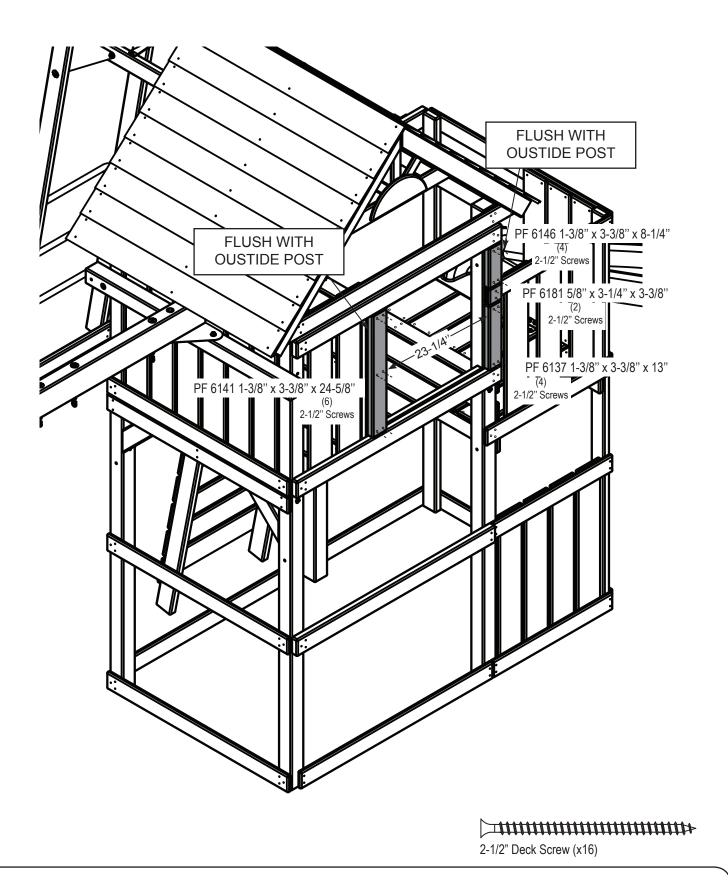
1. Attach Slide Support Boards as shown.
