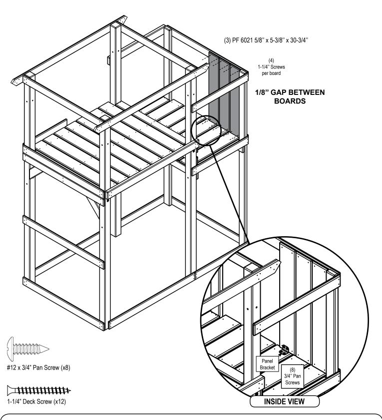
1. Install Barrier Boards as shown.
