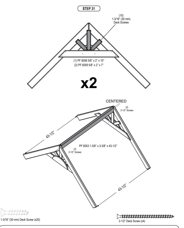
1. Assemble the Roof frame as shown.
