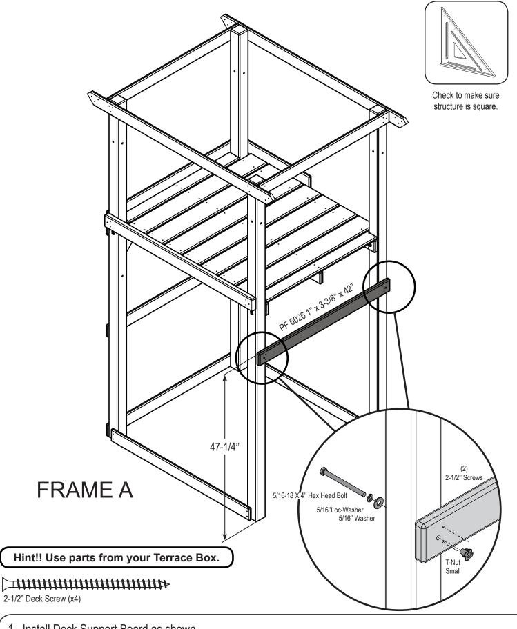
1. Install Deck Support Board as shown.
