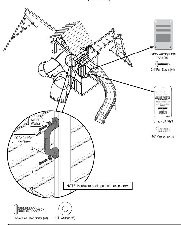
1. Attach Safety Handle, plate and I.D. Tag as shown.
