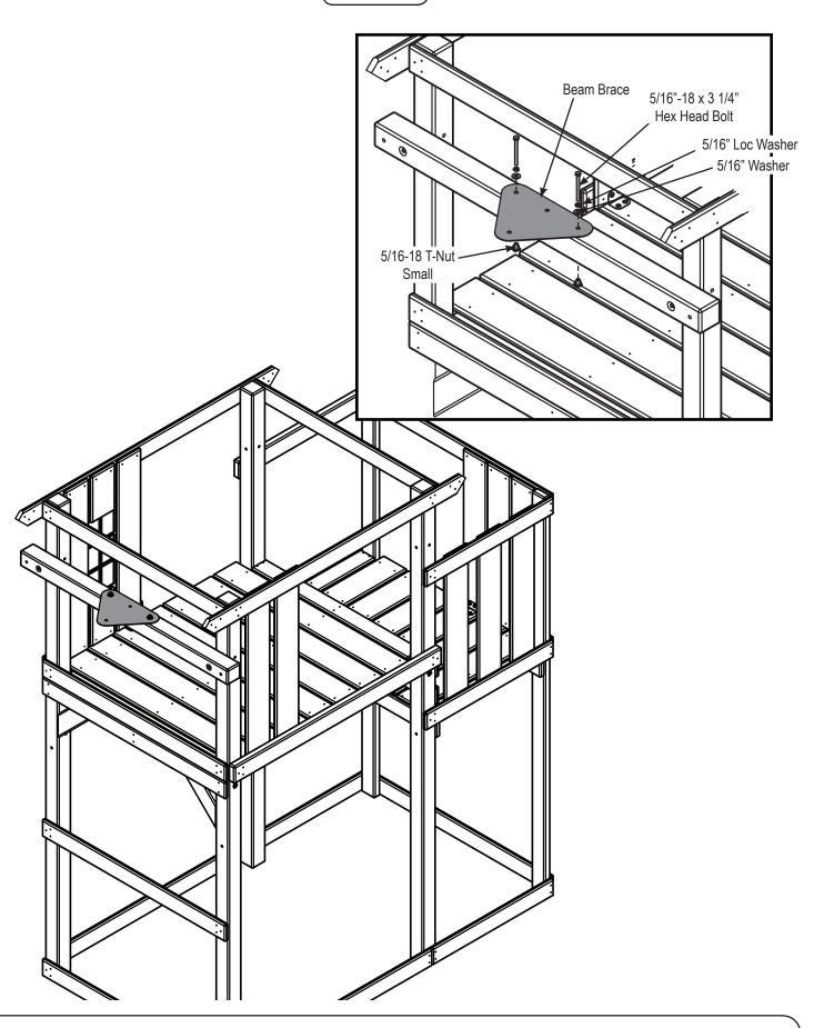
1. Install Swing Beam Brace as shown.
