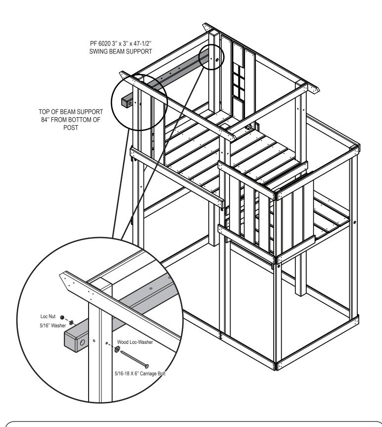
1. Install Swing beam support as shown.
