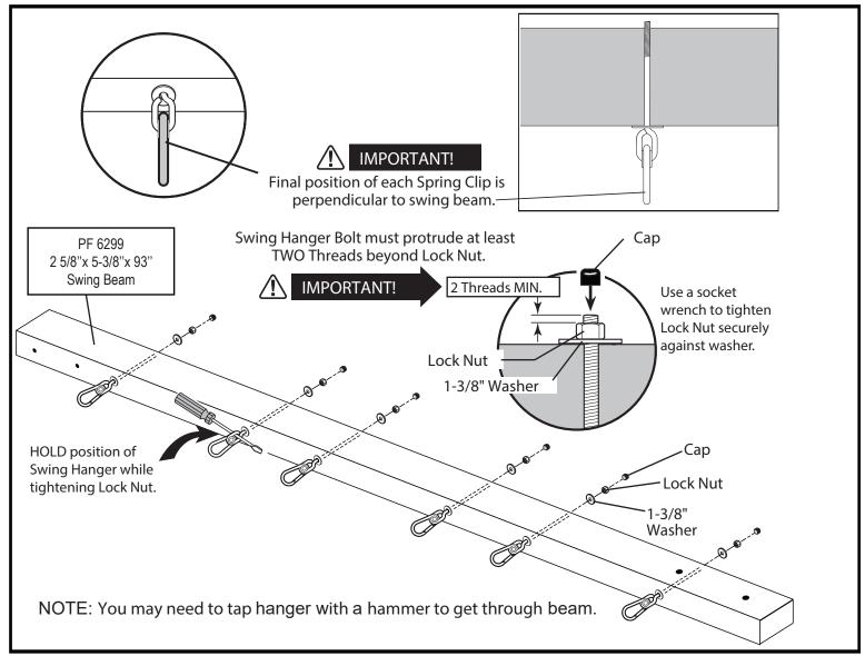
1. Attach Swing Hanger(s) to swing beam as shown.
