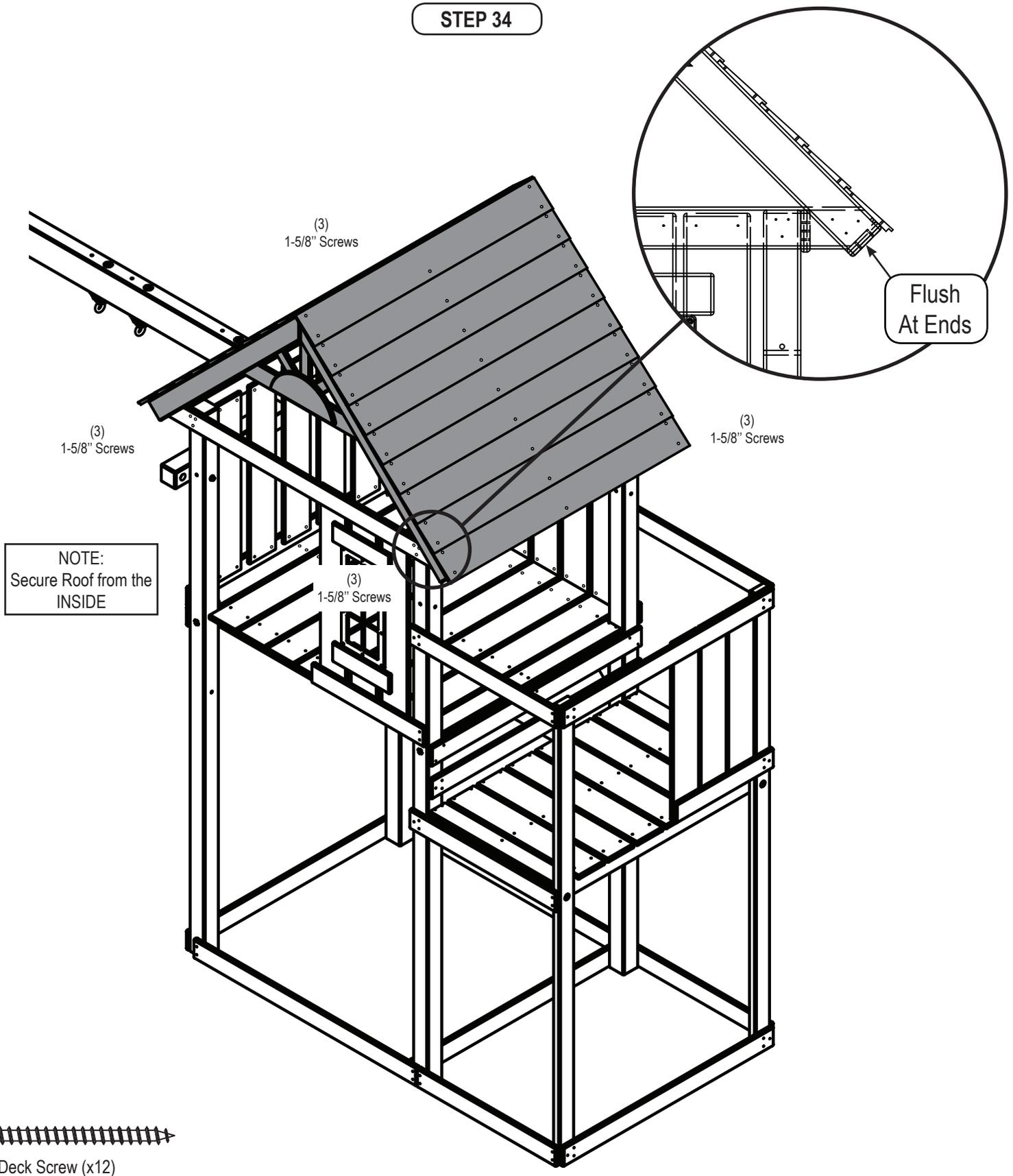
1. Attach Roof Frame to Tower as shown.
