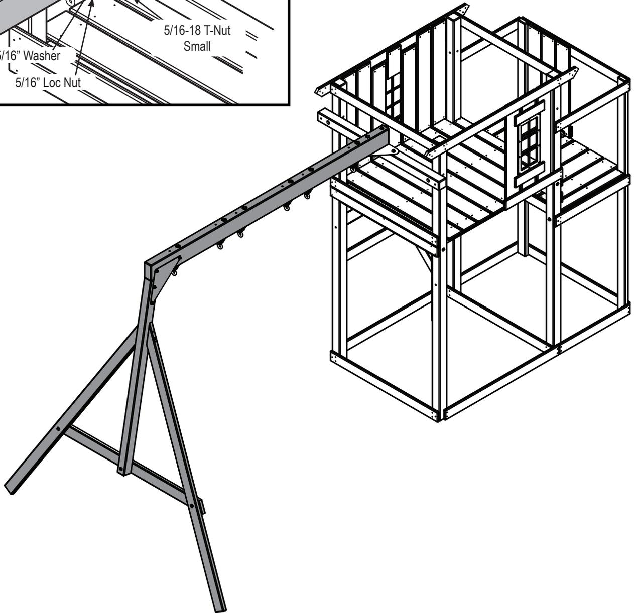
1. Install Swing Beam as shown.
