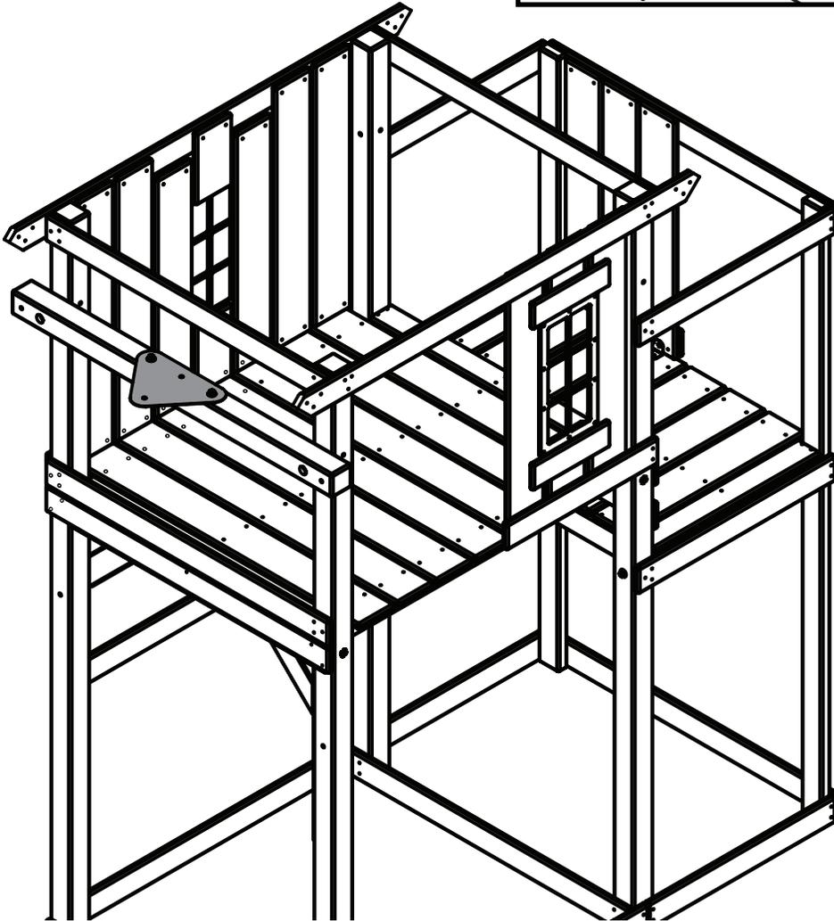
1. Install Swing Beam Brace as shown.
