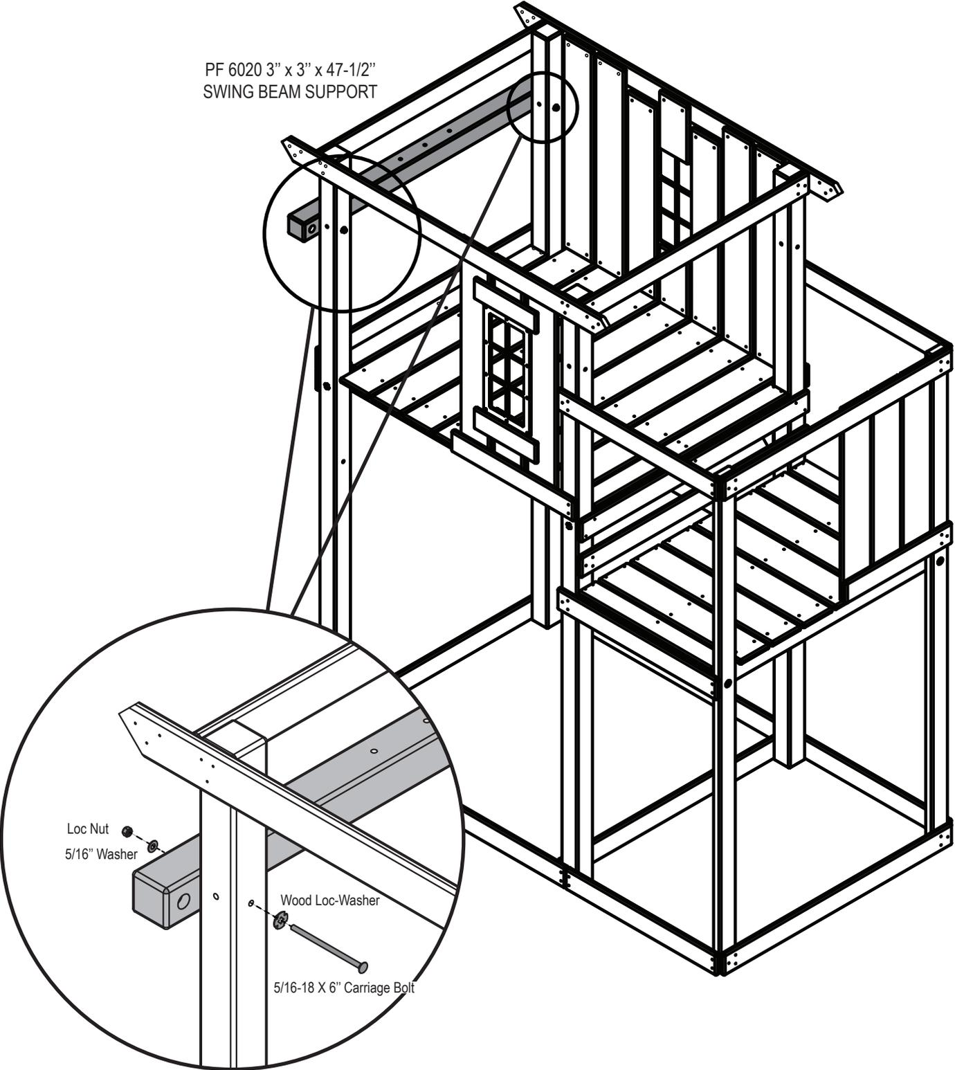
1. Install Swing beam support as shown.
