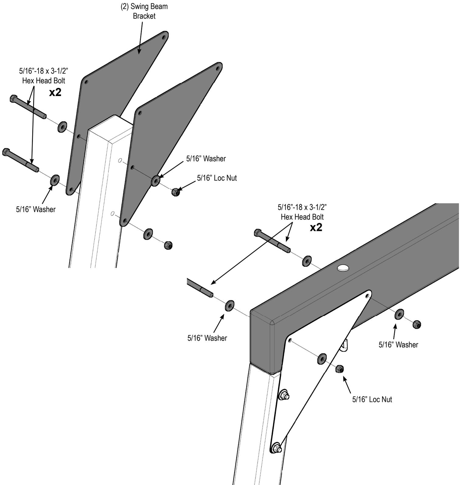
1. Attach Swing Beam Bracket to A-Frame & Swing Beam as shown.
