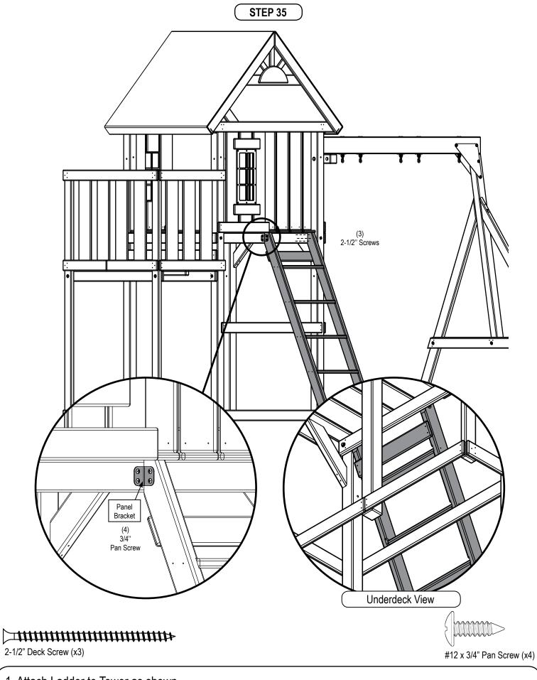
1. Attach Ladder to Tower as shown.
