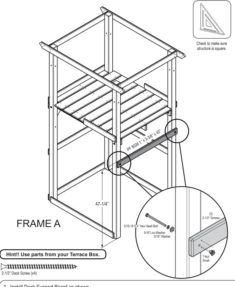
1. Install Deck Support Board as shown.
