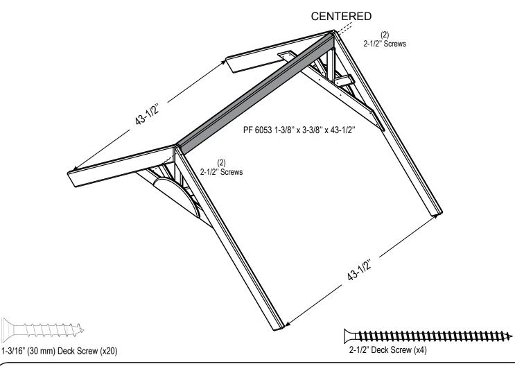
1. Assemble the Roof frame as shown.
