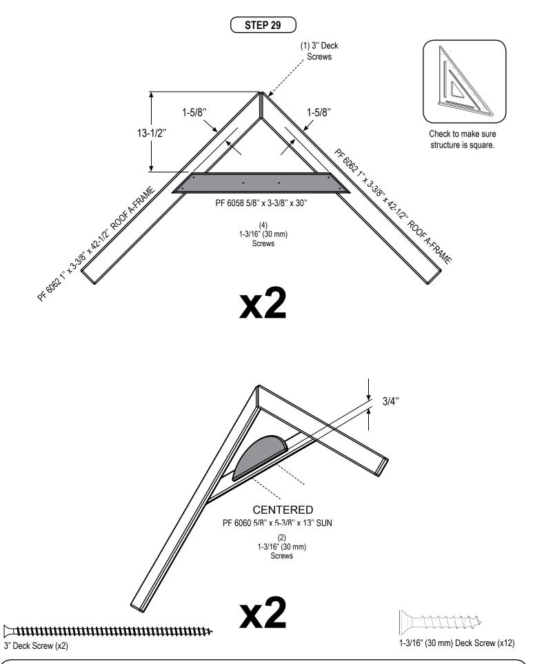
1. Assemble Roof A-Frames as shown.
