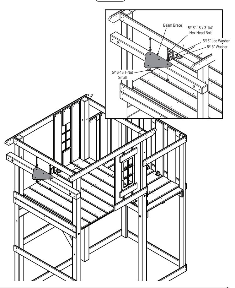
1. Install Swing Beam Brace as shown.
