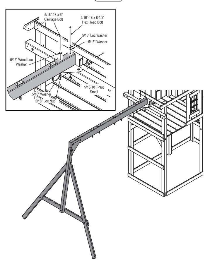
1. Install Swing Beam as shown.
