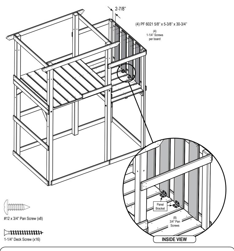
1. Install Barrier Boards as shown.
