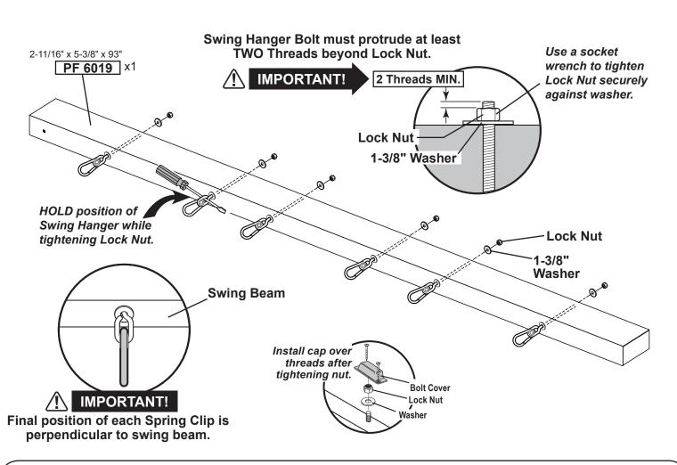
1. Attach Swing Hanger(s) to swing beam as shown.
