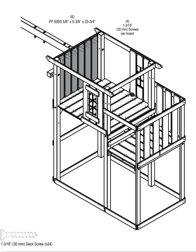
Install Barrier Boards as shown.
