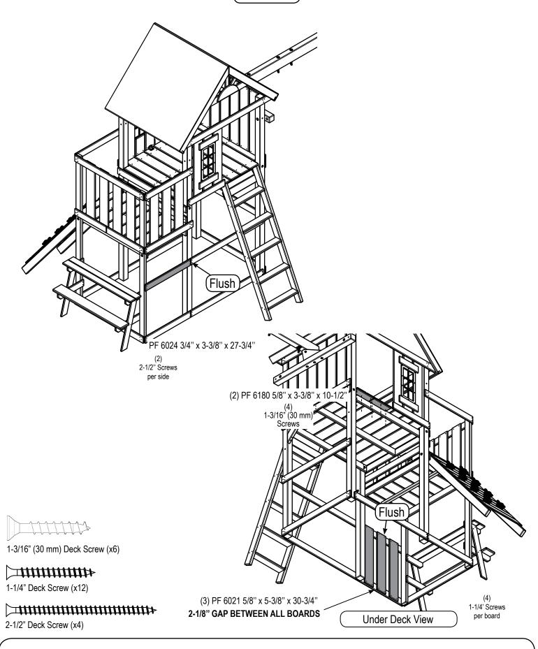
1. Install Barrier Support, Barrier Boards and Slide Support Boards as shown.
