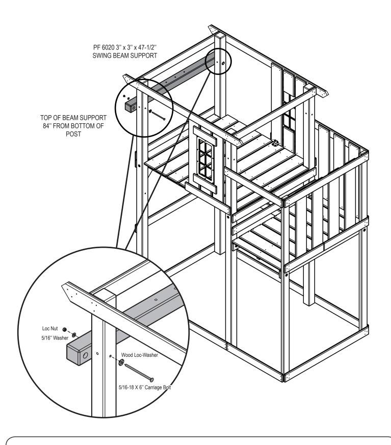
1. Install Swing beam support as shown.
