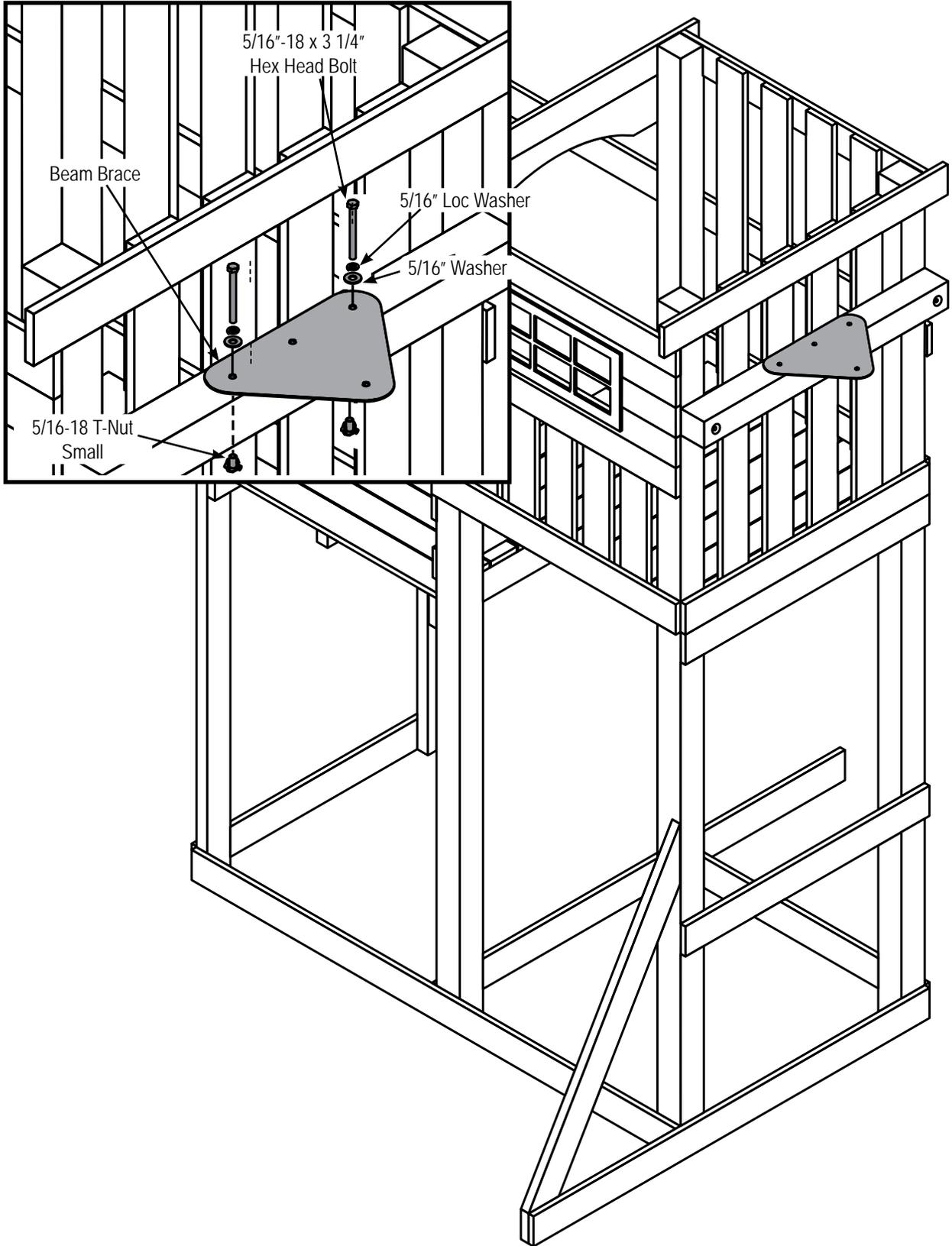
1. Install Swing Beam Brace as shown.
