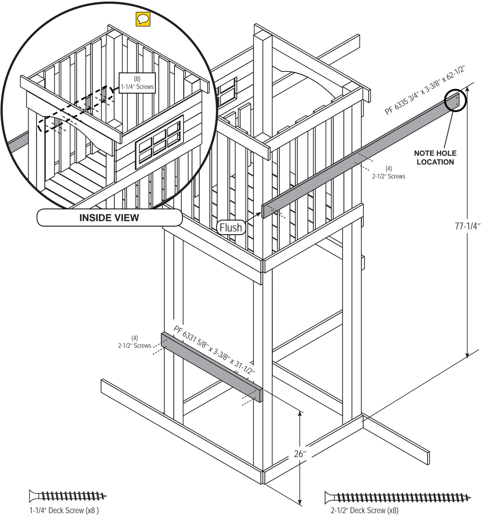
1. Attach Barrier Support Board and Safety Board as shown.
