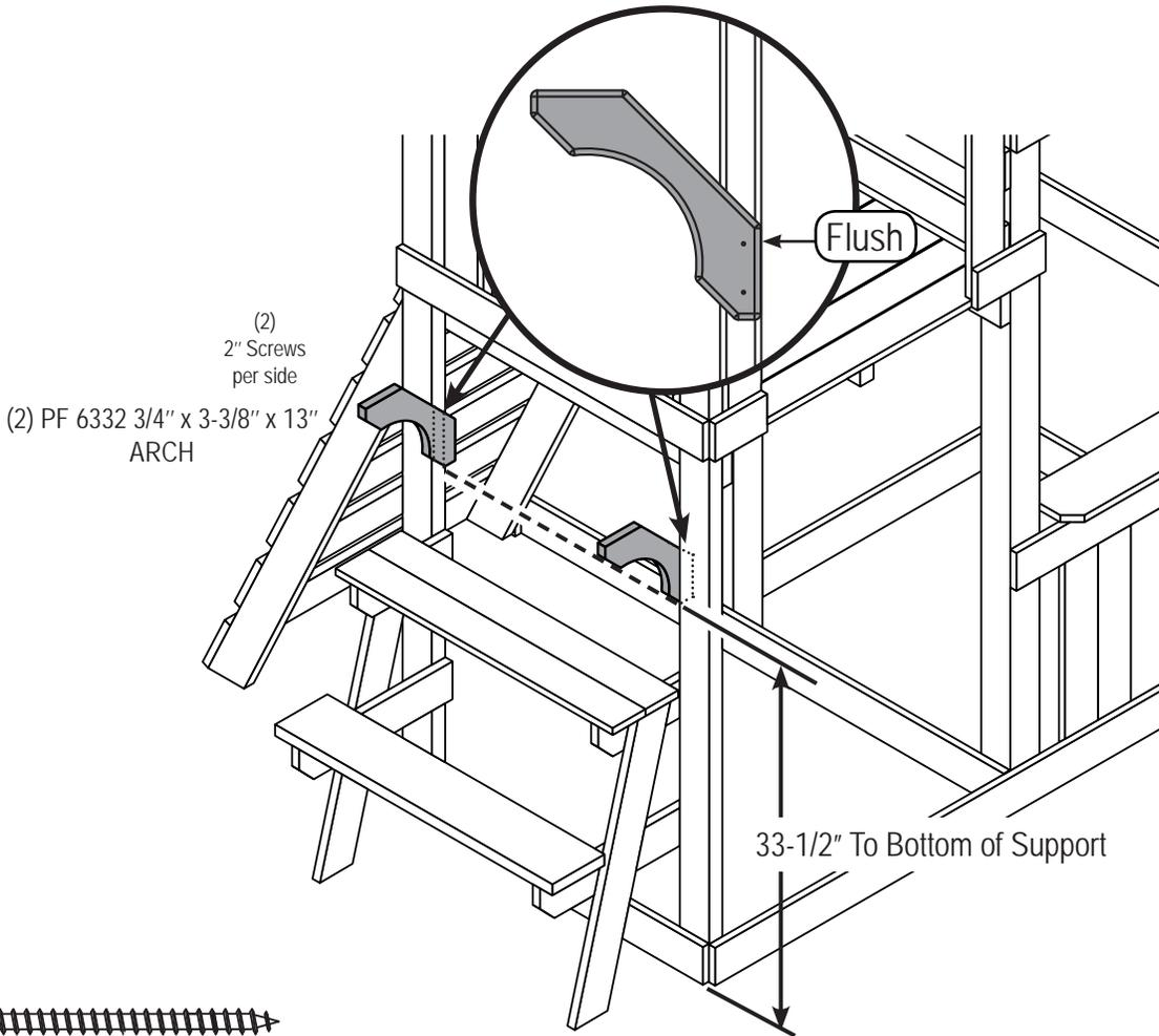
1. Assemble Tarp Frame and Attach Supports to tower as shown.
