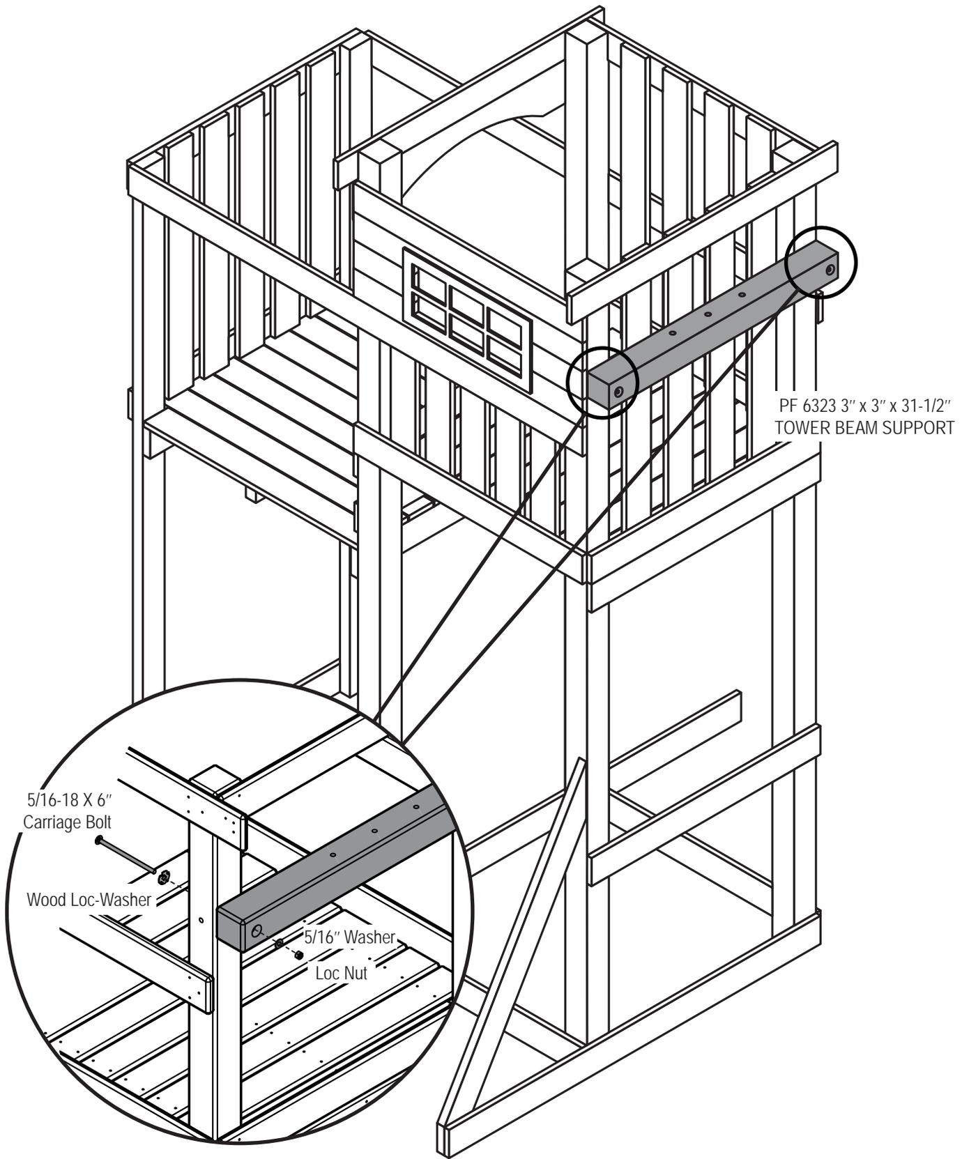
1. Attach Tower Beam Support Board as shown.
