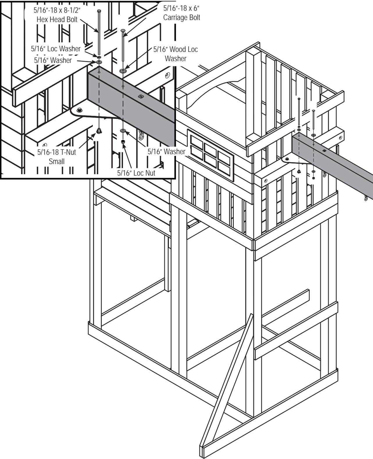
1. Install Swing Beam as shown.
