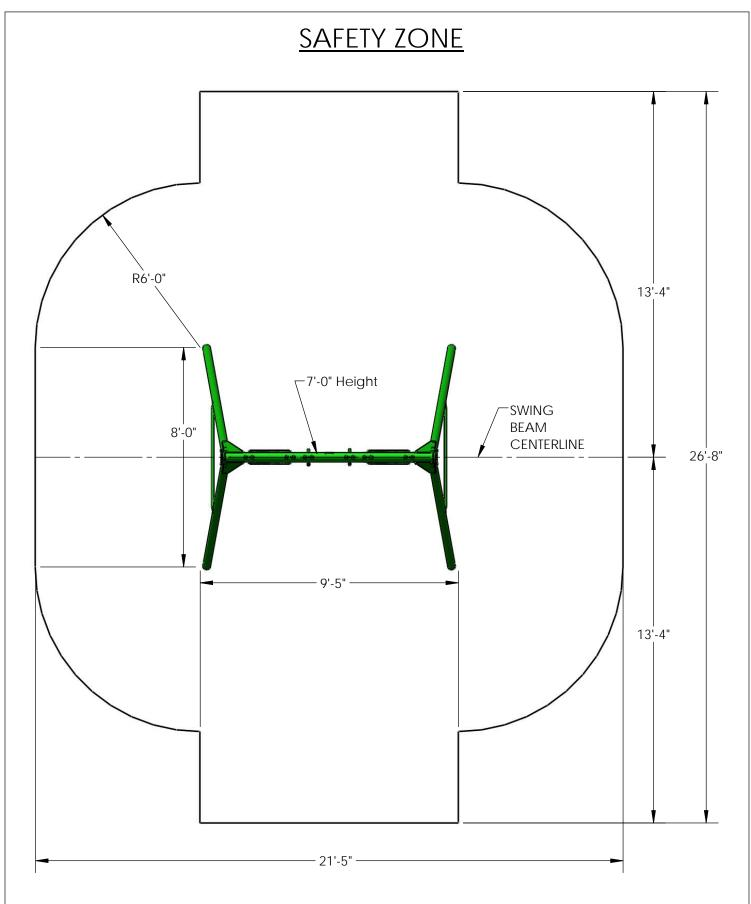
MINIMUM USE ZONE FOR SWINGSET SHALL EXTEND NO LESS THAN 72" FROM ALL SIDES OF THE STRUCTURE. THE SWING USE ZONE SHALL EXTEND NO LESS THAN 13'-4" FORE AND AFT OF THE SWING BEAM CENTERLINE. SWINGS MUST HAVE A MINIMUM CLEARANCE OF 8" ABOVE THE PROTECTIVE SURFACING.
