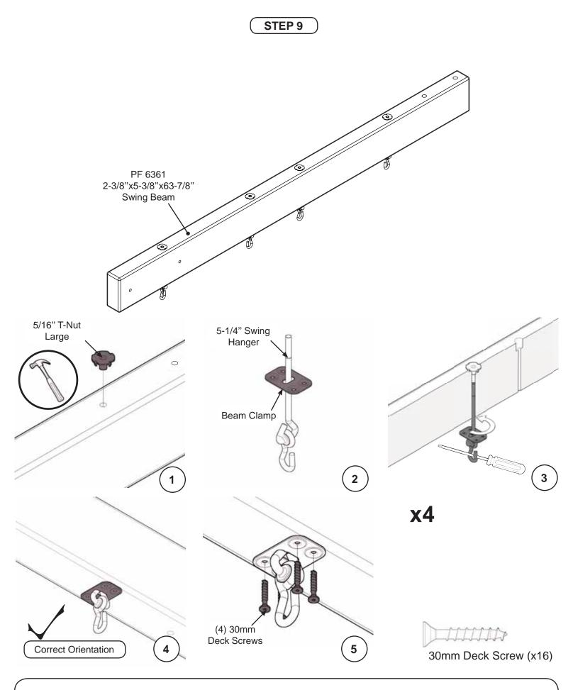
1. Attach Swing Hanger(s) to swing beam as shown.
