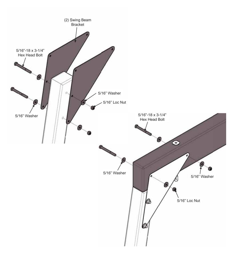
1. Attach Swing Beam Bracket to A-Frame & Swing Beam as shown.
