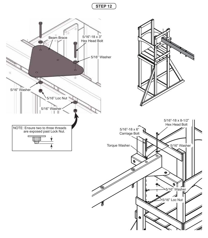
1. Attach Swing Beam to tower as shown.
