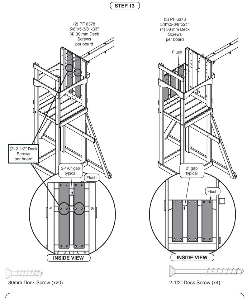
1. Attach barrier boards as shown.
