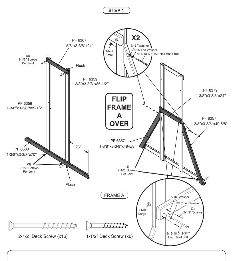
1. Assemble Frame A as shown above. **Note:** Tap each T-Nut into its pre-drilled hole until the metal tangs sink fully into the wood.
